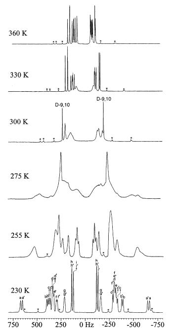
**Figure 3.** 61.4 MHz deuterium NMR spectra for  $1-D_{18}$  in PBLG/CHCl<sub>3</sub> phase as a function of temperature. 208 scans of 3 k data points were added for each spectrum and a recycle delay of 1.5 s was used. Gaussian filtering and zero filling to 16 k data points were employed to improve the spectral appearance and the digital resolution.
